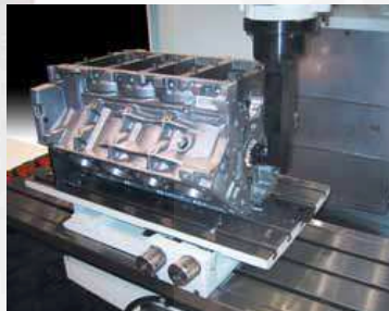
Cam tunnel modifications and roller bearing conversions. Some blocks allow main and cam line to be bored in one set up with extended slim line right angle drive.
