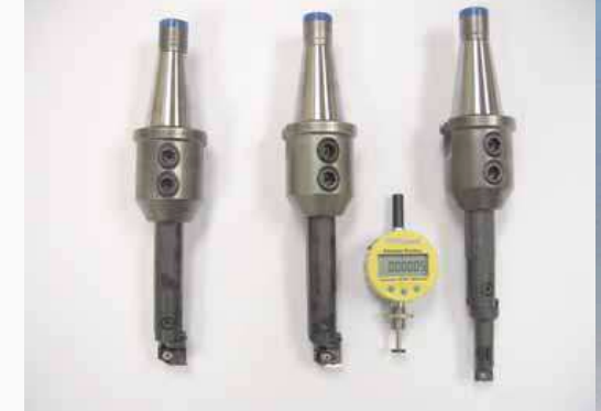
Single point Lifter Tooling and digital setting fixture for boring, facing and finishing lifter bores and bushes.
