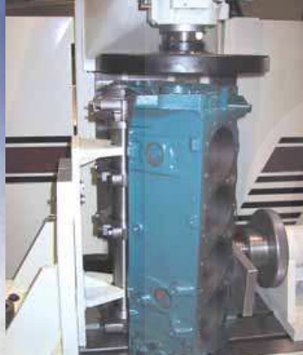
The block end truing fixture quickly attaches to the 4th axis rolover fixture or the precision performance fixture for exact alignment of transmission and engine block. Dowel truing for centralizing transmission and crankshaft centerline
