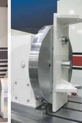
The block end truing fixture quickly attaches to the 4th axis rolover fixture or the precision performance fixture for exact alignment of transmission and engine block. Dowel truing for centralizing transmission and crankshaft centerline
