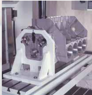
Precision Performance Fixture references from the centerlines of crankshaft and camshaft for machining operations – precise bore locations and square block deck height. Bore and surface a V8 block in less than 30 minutes.
