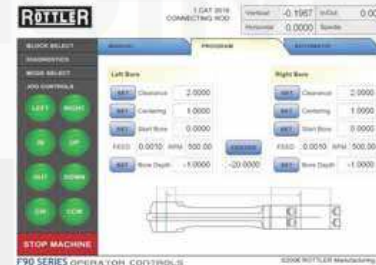
Connecting Rod Touch Screen Control
