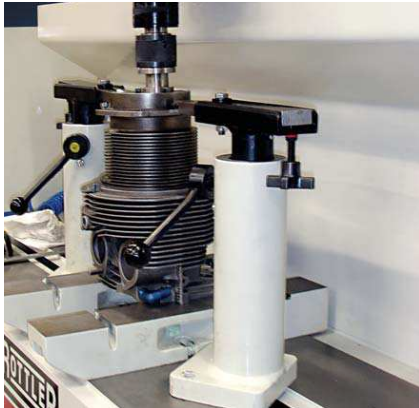
Rottler offers special fixturing for cutting seats in one piece aircraft cylinders. SG 8 only.
