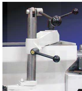
Quick clamp adjustable clamps allow fast clamping of large diesel cylinder heads. SG8 only.
