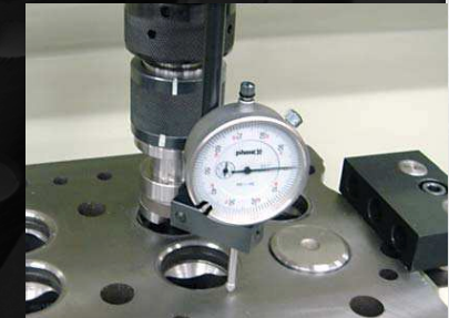
Lower Spindle fixture for depth of cut of the Valve seat. Measured from the head gasket face.
