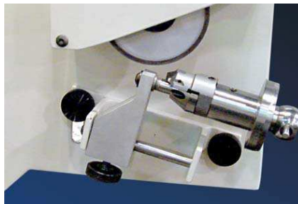
Rottler offers machine mounted tool sharpener for fast easy sharpening of multi-angle tool bits.
