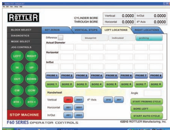
Probe Machine will probe all eight bores and set dimensions for boring. Once finished touch "Start Auto Cycle" to begin boring.
