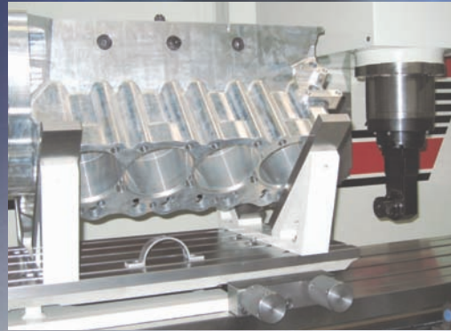
Rottler's new pivot table allows quick set-up for line boring.
