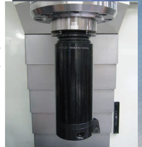
Rottler Boring and Sleeving Cutterhead installed in massive heavy duty F69 Spindle.
