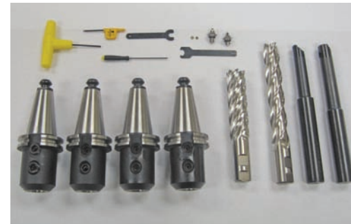
Single point Lifter Tooling fixture for boring, facing and finishing lifter bores and bushes.
