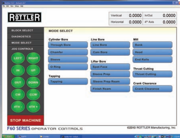
Mode Screen Allows operator to select operation to perform (Select Through Bore).
